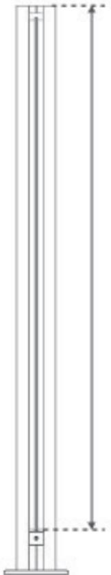
Measure distance between Glass Seating and top of your post. Cut two Glass Sealer strips to this length, one for each side of your glass panel. Repeat for each post.
